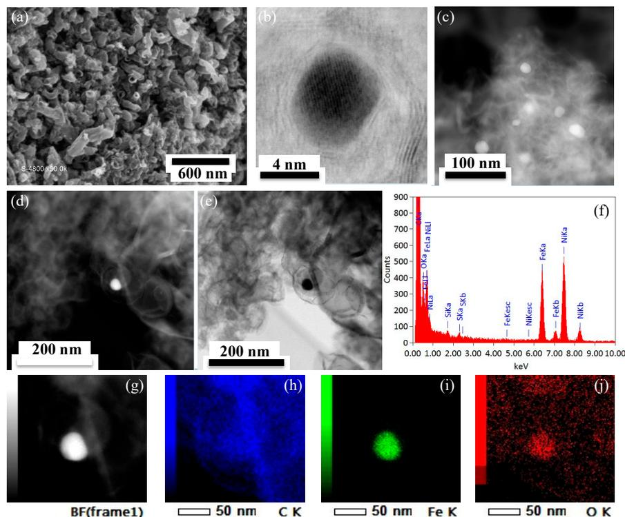
**Figure 6.** (a) Scanning electron microscopy (SEM) image of ICM-FePhen<sub>3</sub>-AW; (b,e) bright-field scanning transmission electron microscopy (BF-STEM) and (c,d) high-angle annular dark-field (HAADF)-STEM images, (f) energy dispersive X-ray spectroscopy (EDX) spectrum measured in the same area as (d) and (e), and (g–j) the corresponding elemental mapping.
