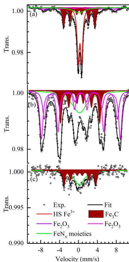
**Figure 3.**  $^{57}\text{Fe}$  Mössbauer transmission spectra and their fittings with spectral components. ICM-FePhen<sub>3</sub> measured at (a) 293 K and (b) 5 K, and (c) ICM-FePhen<sub>3</sub>-AW measured at 293 K.
