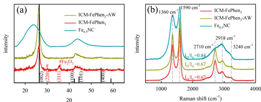
**Figure 2.** (a) X-ray diffraction (XRD) patterns, and (b) Raman spectra of ICM-derived Fe-N-C catalysts. The XRD and Raman spectra of Fe<sub>0.5</sub>NC (a ZIF-8 derived Fe-N-C pyrolyzed material [11]) are also presented as references for a material that comprises only FeN<sub>x</sub> moieties integrated in amorphous carbon.
