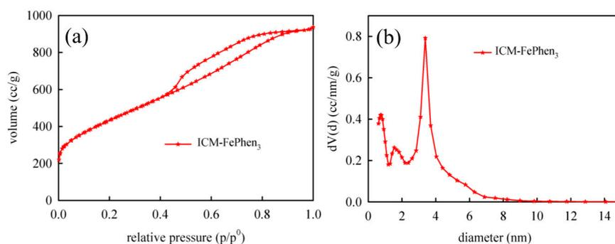
**Figure 5.** (a) N<sub>2</sub> adsorption/desorption isotherm, and (b) the corresponding pore size distribution from density functional theory (DFT) method of ICM-derived Fe–N–C catalysts.
