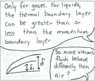
Precisely! This leads us to a dimensionless number, the Prandtl Number.  $Pr^{\frac{1}{3}} = \frac{8}{8r} = \left(\frac{V}{A}\right)^{\frac{1}{3}}$  V = momentum diffusivity A = thermal diffusivity Pr = Prandtl NumberWoah.
