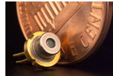
Visible Red Laser diode AlGaInP
