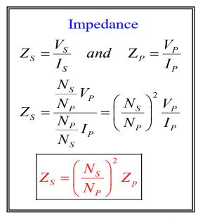
Function generator  $Z_P = 50\Omega$ Speaker  $Z_S = 8\Omega$ Voltage Divider  $V_S = V_{FG} \left( \frac{Z_S}{Z_S + Z_{FG}} \right)$  $= V_{FG} \left( \frac{8\Omega}{8\Omega + 50\Omega} \right)$  $V_S = V_{FG} / 7$  only 14% gets to speaker
