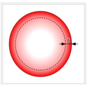
Distribution of current flow in a cylindrical conductor, shown in cross section. For alternating current, most (63%) of the electric current flows between the surface and the skin depth, δ, which depends on the frequency of the current and the electrical and magnetic properties of the conductor.
