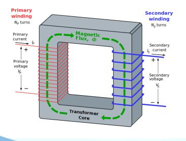
Current in coil produces B - field  $B_N = \mu_o \eta I$  for  $\eta$  turns / length Now assume  $\eta = N$  (L is fixed) B - field produces magnetic flux  $\Phi = B_N A$  A = areaVoltage (EMF) produced by change in flux  $V = -N d\Phi / dt$  for primary  $V_S = -N_B d\Phi / dt$  for primary  $V_S = -N_S d\Phi / dt$  for sec ondary Suppose  $N_S$  catches all the  $N_P$  flux  $V = \frac{N_S}{V}$  looks like gain  $G = \frac{N_S}{V}$
