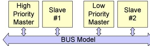
Fig. 6. Dual master setup for accuracy measurements.
