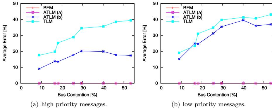
Fig. 17. Individual timing accuracy for the CAN models.
