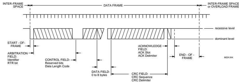
Fig. 15. CAN Data Frame (Source [Philips ]).
