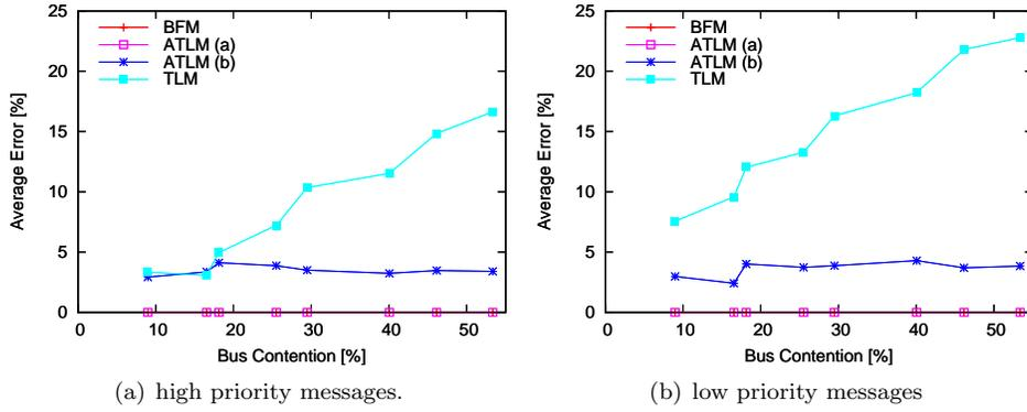
Fig. 18. Cumulative timing accuracy for the CAN models.
