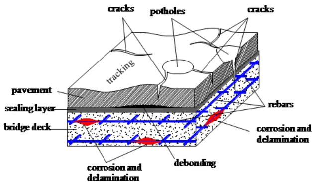
**Figure 1: Some common defects and deteriorations found in concrete bridge decks with asphalt pavement overlay**
