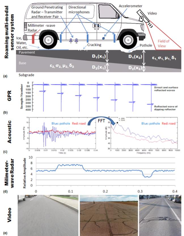
**Figure 2:** (a) Schematic of VOTERS roaming sensor system (van) equipped with an access point and multi-modal sensor systems. They collect data streams sensing roadways for surface and subsurface defects, layer thickness, and properties. Four different types of data (3.1.1) are collected: (b) GPR traces, (c) acoustic waves, (d) millimeter-wave radar, and (e) video images.
