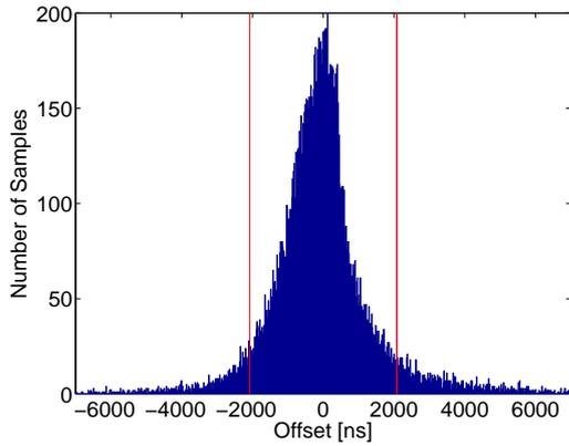
Figure 7: Results of Software-based Timing Synchronization
