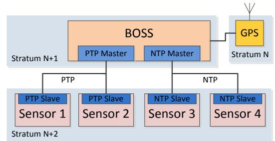
Figure 6: Software-based Timing Synchronization
