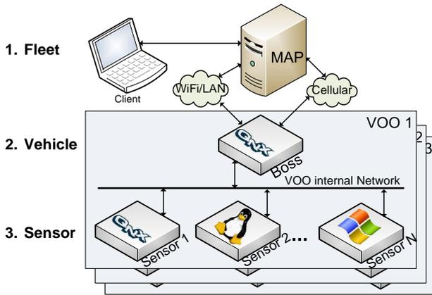
**Figure 3: Multi-Tiered Communication Architecture**
