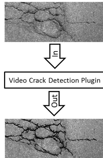
Figure 10: Example Crack Detection Plugin operating on Black and White video image input stream and creating binary image data stream of detected cracks and a text file containing statistics on the detected crack classes, e.g. 326673 total pixels, 1171 pixels or 0.36% transverse cracks, 76 pixels or 0.02% longitudinal cracks, 1201 pixels or 0.37% transverse cracks, and 2448 pixels or 0.75% diagonal cracks [14].
