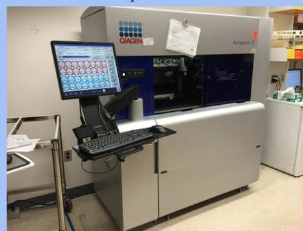
Figure 1. This is the autopure LS machine that is used to automatically extract DNA from blood samples.
