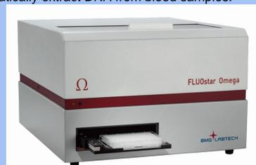
Figure 2. This is the FLUOstar Omega machine that we use for DNA quality control. We use this to measure DNA quantification by using fluorescent dye to distinguish between RNA and other proteins.
