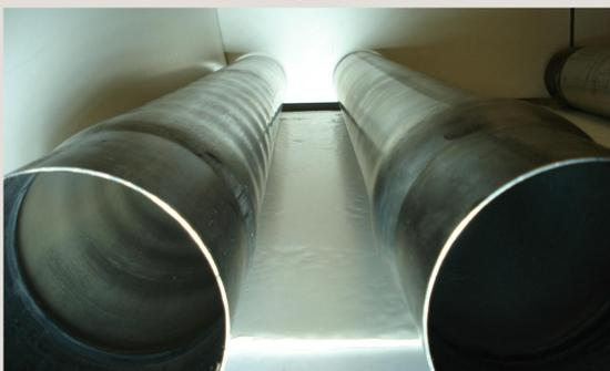
Figure 1: Unprotected tubes after detonation.
