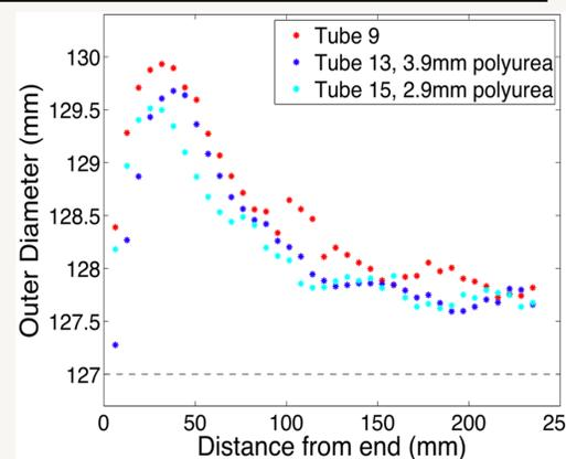
Figure 2: Plastic strain from 2-bar detonation.
