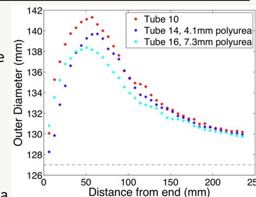
Figure 3: Plastic strain from 3-bar detonation.
