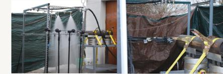
Water Spray Test Set-Up
