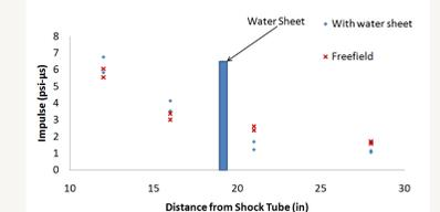
Free Field Vs. Water Sheet, Peak Overpressure and Impulse
